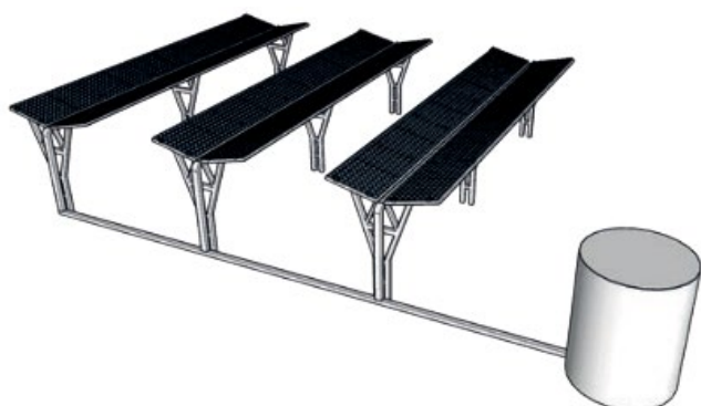
Figure 6 - Concept design for a rainwater harvesting system with storage tank
